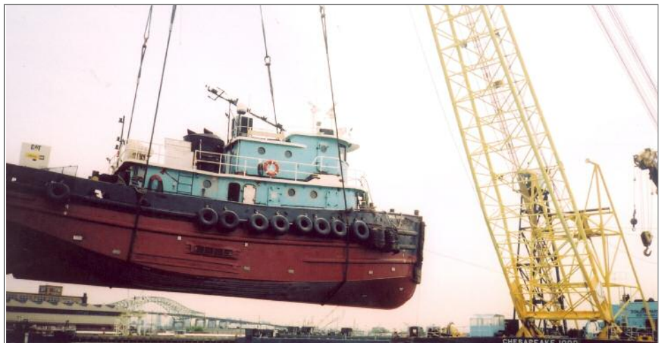
No drydock needed; Donjon’s Chesapeake 1000 picks up the Brian Nicholas to be placed onto a Donjon barge.
