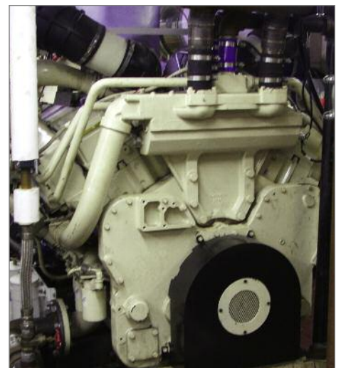
The heart of the rebuild, K38-M Tier 2 main engines.
